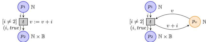
Fig. 3. Global variable notation (left) and corresponding semantics (right)
