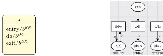
**Fig. 4.** A simple state (left) and its translation (right)
