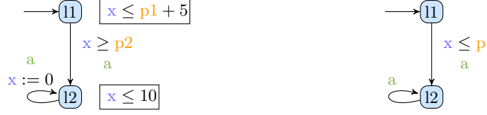
(a) PTA deadlocked for some valuations (b) PTA deadlocked for all valuations
